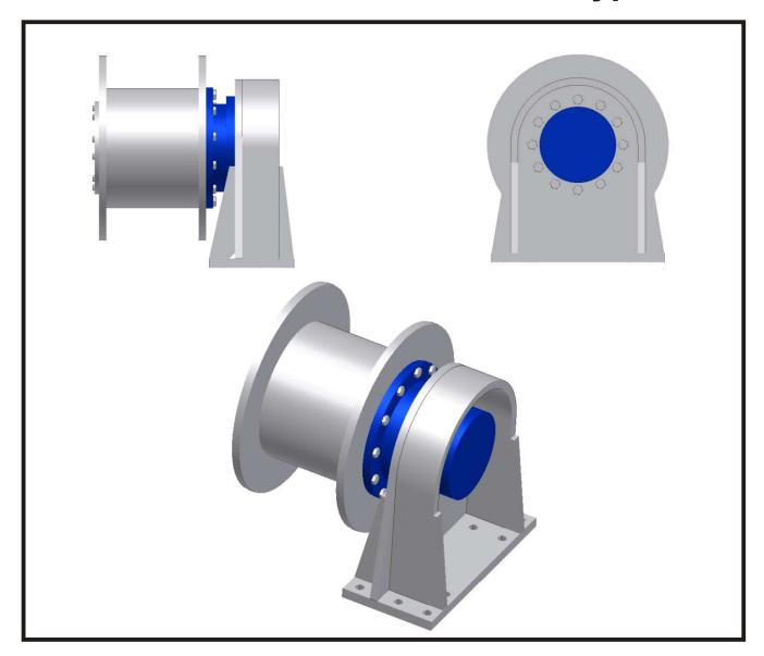
The winch is made out of steel. Surface treatment includes: Sand blasting, metallisation, coating and paint. The winch is hydraulic with an hydraulic motor and planetary wheel drive fitted directly onto the drum. The winch has a simple design and is durable, it therefore requires very little maintenance.
